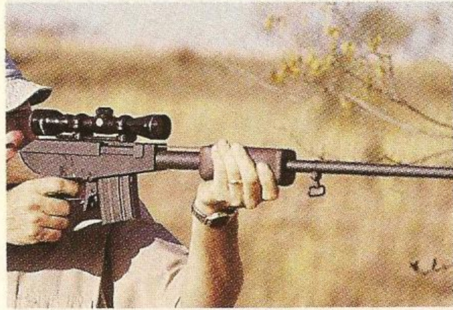
Without doubt the most unusual transmutation of an infantry rifle in the history of military small arms, the Vektor H5 is a commercial, slide-action version of the gas-operated, selective-fire R4. Photo: courtesy LIW
